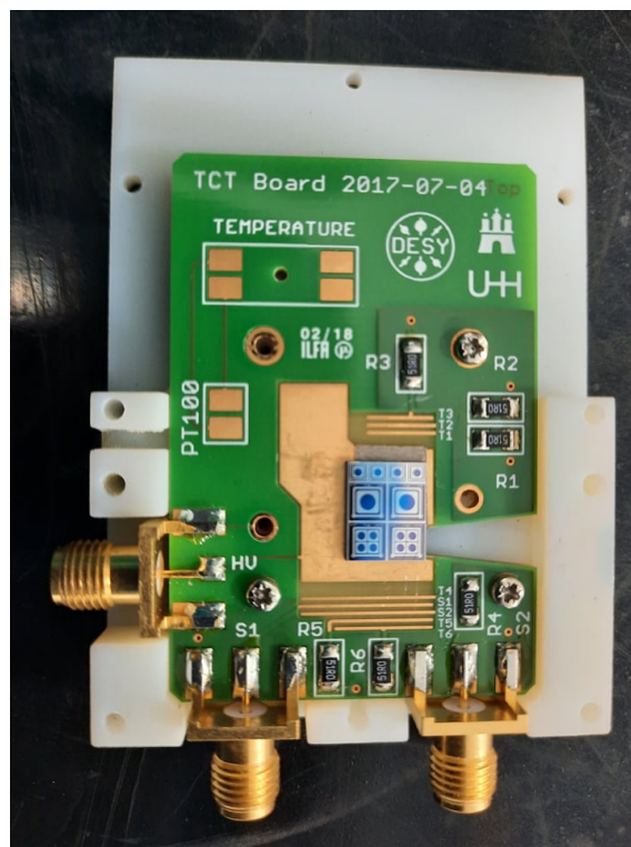
Figure 3.19: The PCB used for TCT measurements. The board supports dual-channel readout where the resistors work with the parasitic capacitance built into the PCB to filter DC, similarly to the bias-T. However, it is primarily used in a simple single-channel readout which requires no electronics on the PCB.
