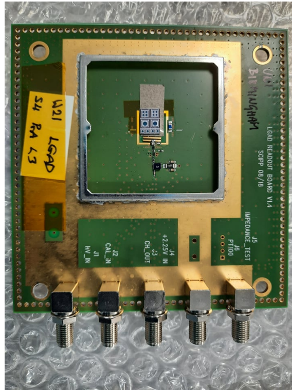
Figure 3.26: Developed by the University of Santa Cruz, this PCB is used for time resolution measurements [46].
