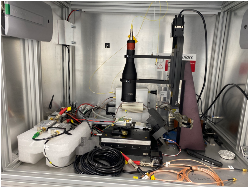
Figure 5.18: Gain setup, including the laser, beam monitor and the LGAD on a mechanical stage.
